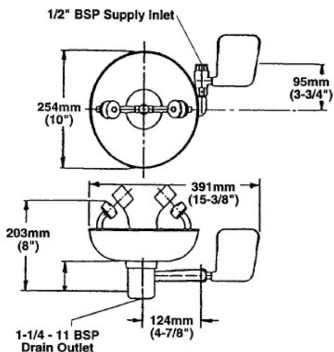
NOTE: The top of the eyewash heads should be positioned 1067mm (42") from floor
