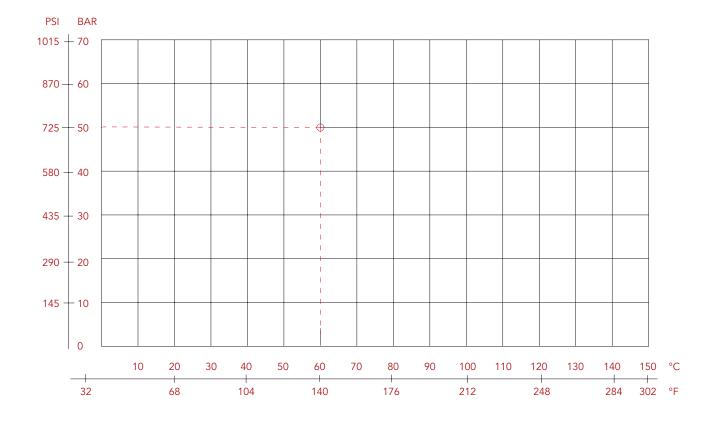
NB: Maximum working temperature for gas: +60 °C The working pressure for gas is from 0 to 5 bar.
